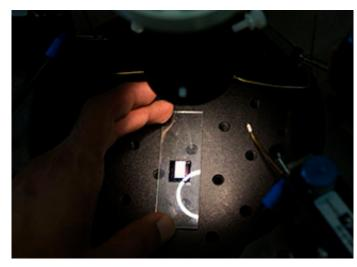
Girish Kulkarni, Electrical Engineering PhD Student, runs an experiment testing the vapor sensors that he has helped develop as part of a collaboration between Xudong Fan, BME Professor, and Zhaohui Zhong, EECS Professor, in the LBME Building. The sensors allow for the measuring of different vapors, whereas other sensors can only read for one type of vapor. Photo: Joseph Xu, Michigan Engineering Communications & Marketing
