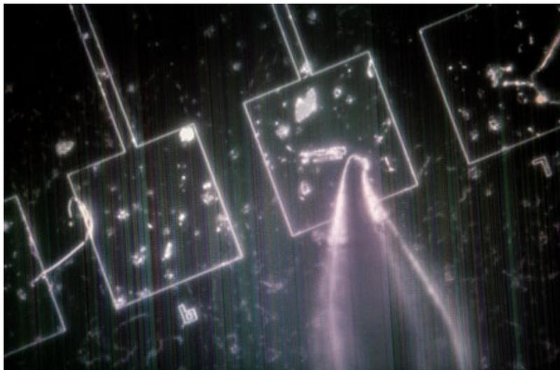
*A magnification of the sensor. The sensors allow for the measuring of different vapors, whereas other sensors can only read for one type of vapor.*
